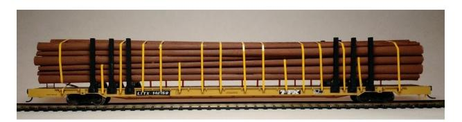
After completing this scratch built HO scale 89' LTTX flatcar, it was time to create a prototypically accurate load of utility poles for the car to carry.
